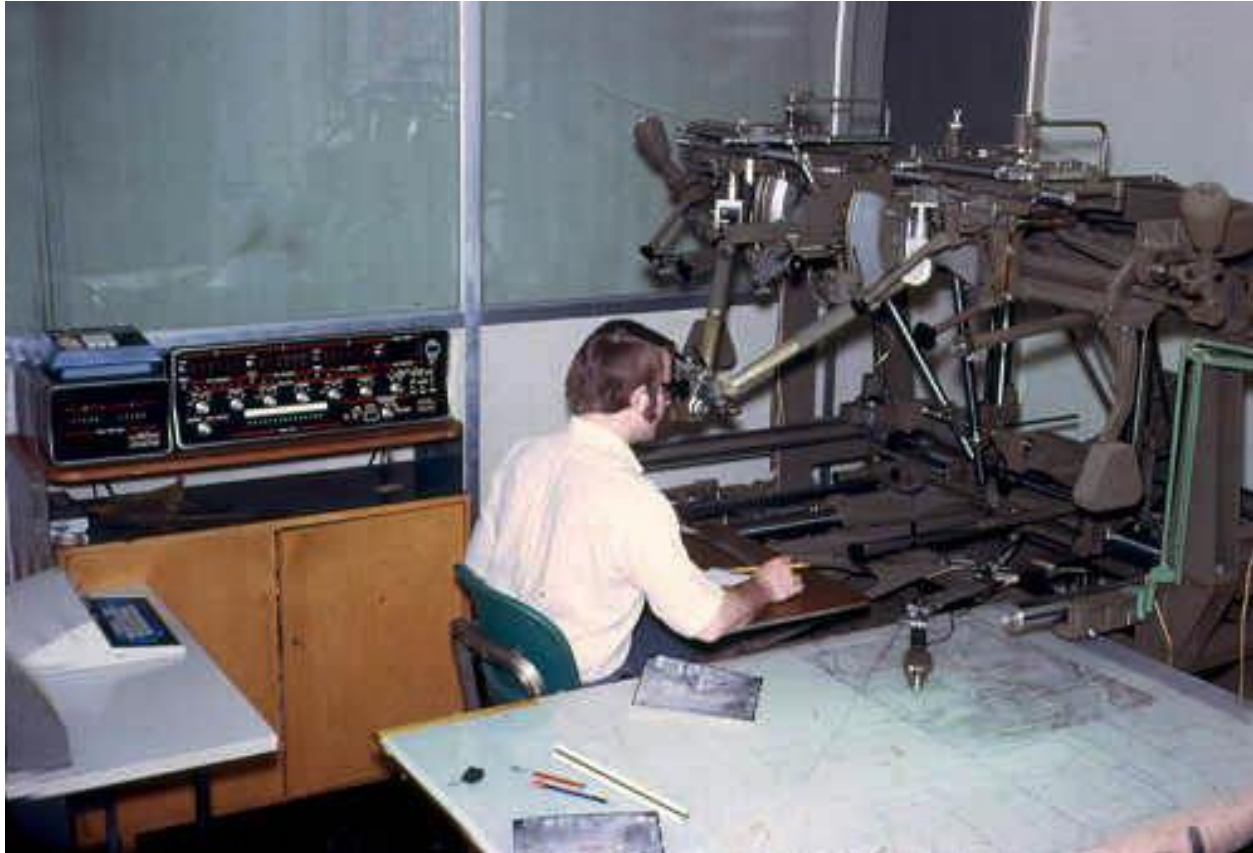
Galileo Santoni model III analog stereoplotter. Photo by W. Mayo
